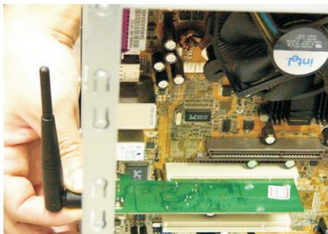
Note: Please make sure that antenna is tightly screwed to get optimal receiving coverage area.
